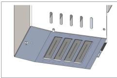
Printing heads are spring loaded and protected with a stainless steel 1.5mm thick skid to protect them from accidental strikes
